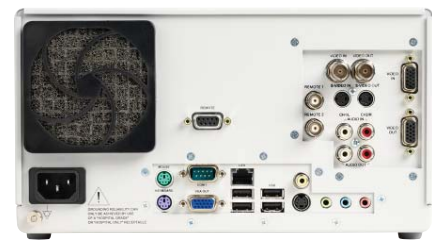
MEDICAL DVD RECORDER, S-VIDEO INPUT TO MPEG OUTPUT
